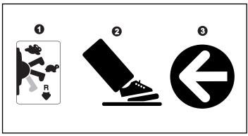
Please Note: To avoid damaging the motors and gears, stop the vehicle before shifting from forward to reverse ( ).
